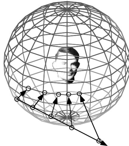
Fig. 1. Schematized sound source path relative to the spherical projection surface of a binaural receiver (listener).
