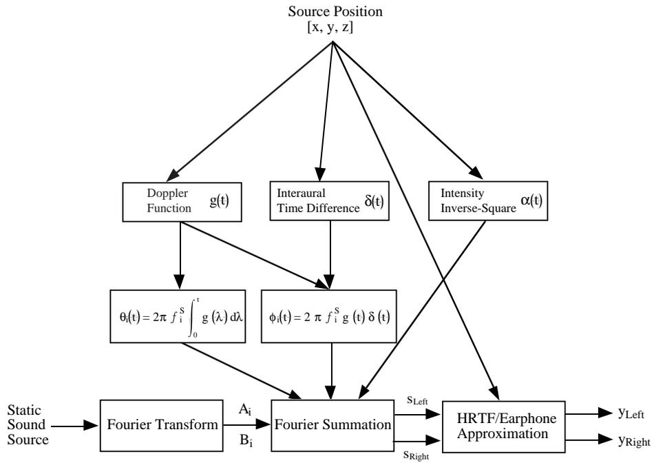
Fig.4. Schematic of virtual 3D auditory motion synthesis.
